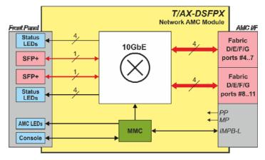
Functional Block Diagram  $\underline{\text{of T/AX-DSFPX}}$  Network AMC-module
