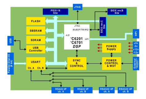
*TORNADO-E62/E67* are ultra-high performance embedded DSP controllers with the industry standard 3U form-factor for real-time data acquisition and DSP. Flexible modular construction and a variety of "off-the-shelf" AD/DA/DIO and I/O coprocessor expansion daughter card modules make *TORNADO-E62/E67* an ideal selection for embedded telecommunication, telephony, multimedia, acoustics, instrumentation, digital radio and many more application.
