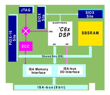
TORNADO-62MX/67MX is an ultra-high performance and low cost DSP platform with compact industial MicroPC® form factor, which installs into any industrial ISA-bus host computer into 8-bit ISA slot. Flexible modular system architecture and a variety of AD/DA/DIO/Coprocessor expansion daughter card modules make TORNADO-62MX/67MX an ideal selection for telecommunication, telephony, multimedia, acoustics, instrumentation and digital radio applications in industry.
