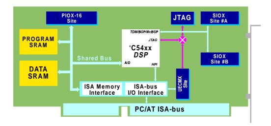
TORNADO-548/549/5402/5410/5416 are high performance DSP platforms for real-time DSP and universal TMS320 DSP emulators for ISA-bus host PC. Flexible modular construction and a wide selection of AD/DA/DIO expansion daughter-card modules make TORNADO-548/549/5402/5410/5416 an ideal selection for telecom, telephony, speech/fax/modem, audio, instrumentation and biomedical application as well as for OEM, education and TMS320 DSP systems development and diagnostics.
